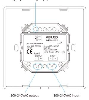
Select leading edge(forward-phase) dimmer or trailing edge(reverse-phase) dimmer according to dimmable LED light or driver.
