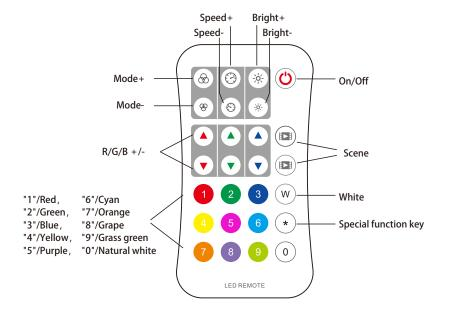
Mode+/-: Short press switch dynamic mode builtin controller
